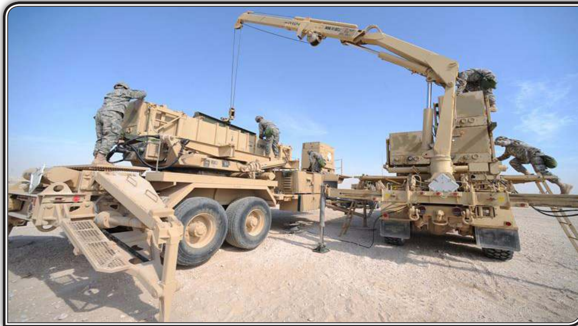
Army Patriot Launch Station operators/maintainers from Bravo Battery, 1-43 Air Defense Artillery, perform a guided-missile transporter reload certification at an undisclosed Southwest Asia location, Feb. 12, 2010.
